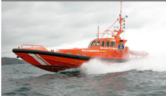
55 IMMEDIATE SAR UNIT Fast intervention unit. Up to 400miles LOA = 21m
