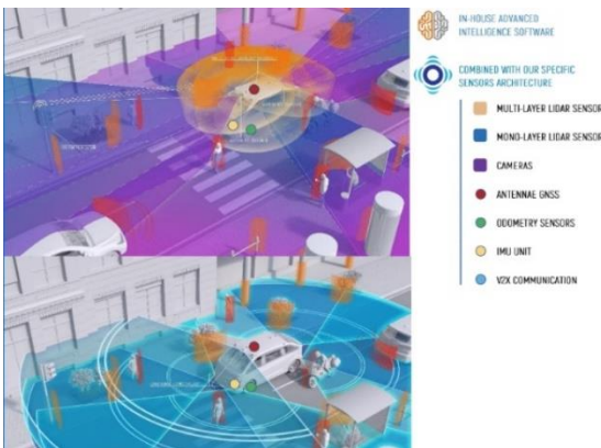
Fig. 4 Cutting-edge multi-sensor technology Source: Navya Safety Report 2019
